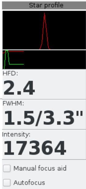
This tool is to control the focus by examination of a star image. It can be used with a manual or motorized focuser.
