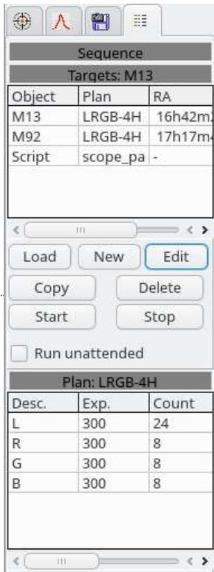
This tool is to control a complex sequence of exposure on one or more objects.
