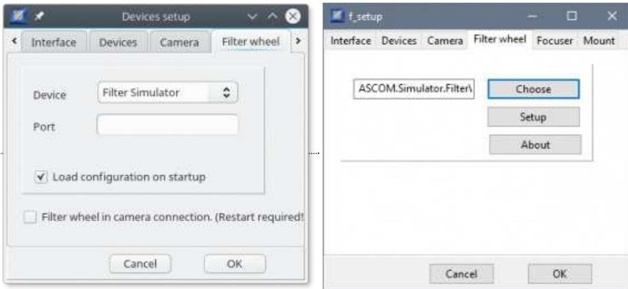
Select the filter wheel to use with CCDciel, from the dropdown list for INDI or using the ASCOM chooser. Or check the corresponding box if the filter wheel is commanded by the camera driver.
