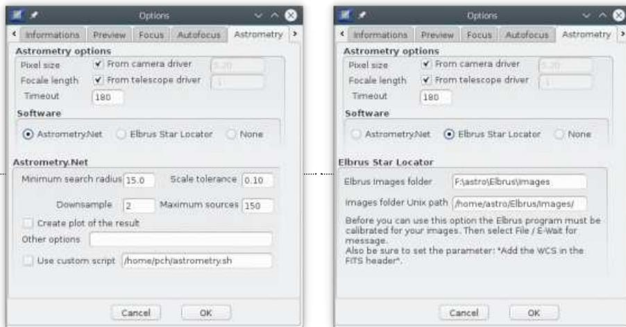
Enter the camera pixel size and telescope focal length, or if applicable for your driver, check the box to get it automatically.
