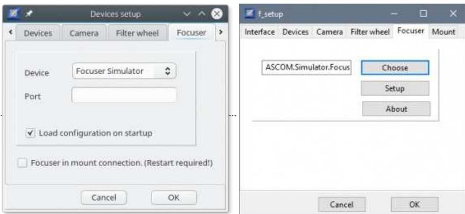
Select the focuser to use with CCDciel, from the dropdown list for INDI or using the ASCOM chooser. Or check the corresponding box if the focuser is commanded by the mount driver.
