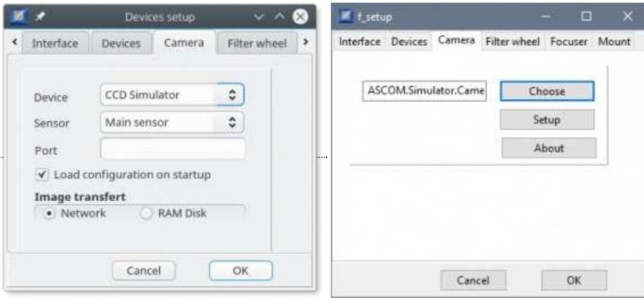
Select the camera to use with CCDciel, from the dropdown list for INDI or using the ASCOM chooser. For INDI the “sensor” field is to select the sensor to use for dual-chip camera, you probably always want “Main sensor” here.
